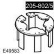
Rear wheel bearing remover/installer 205-802/5
